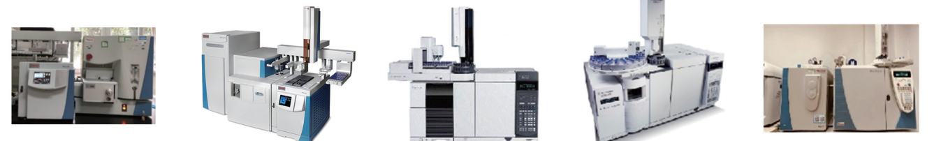
三重四极杆-气质联用仪 Thermo Trace 1310 TSQ Quantum XLS 高分辨气相色谱质谱联用仪 Thermo Q Exactive GC 单四极杆-气质联用仪 Agilent 7890B-5977B 单四极杆-气质联用仪 Agilent 7890A-5975C 单四极杆-气质联用仪 Thermo Trace GC ULTRA-DSQ II
